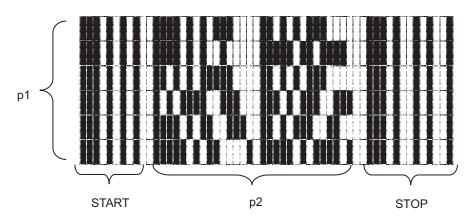
PDF417 is configured by a fixed bar pattern for starting and stopping, and a bar pattern called a code word. Code words are configured by 17 modules.
