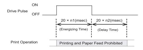
Drives for external buzzers set using this command is performed by <ESC> <GS> <EM> <DC2> m n1 n2.
